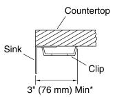
\* Allow clearance around sink rim for clip attachment.
